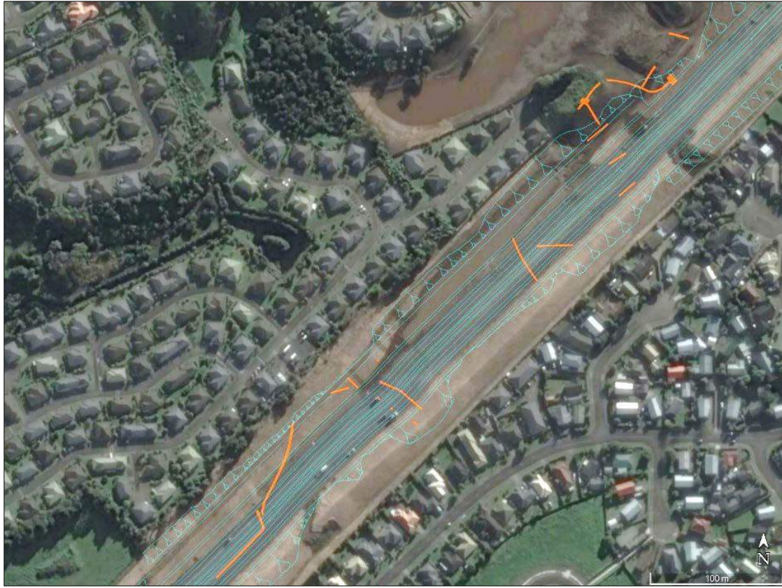
Figure 9. Aerial view of northern section of Sector 2 showing location of trenches. The blue lines indicate the proposed cut and fill for the construction of the road.
